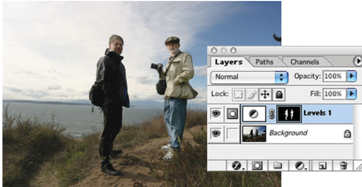
FIGURE 14.11 Our camera’s matrix meter favored the sky in this image, resulting in the foreground figures being overexposed. (To avoid this problem, we should have used the camera’s center-weight meter.)
